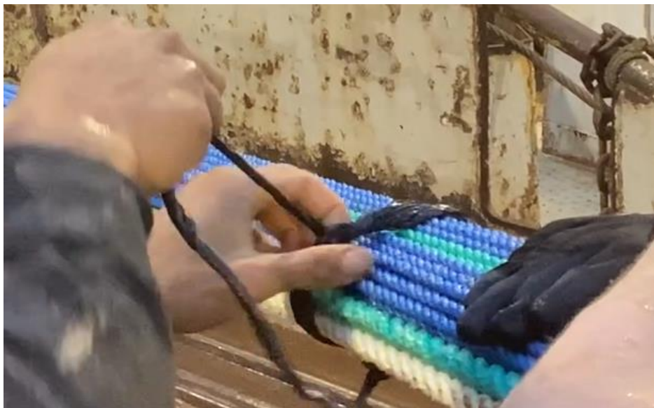
Figure 5: binds loop around the trawl meshes, then a few slip hitches applied
