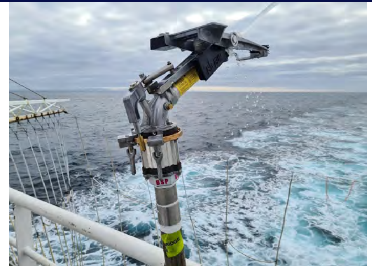
High-capacity water sprayer deployed from the fantail of FV Tokatu in trial to deter seabirds from the area during hauling of the trawl. Image: Sealord
