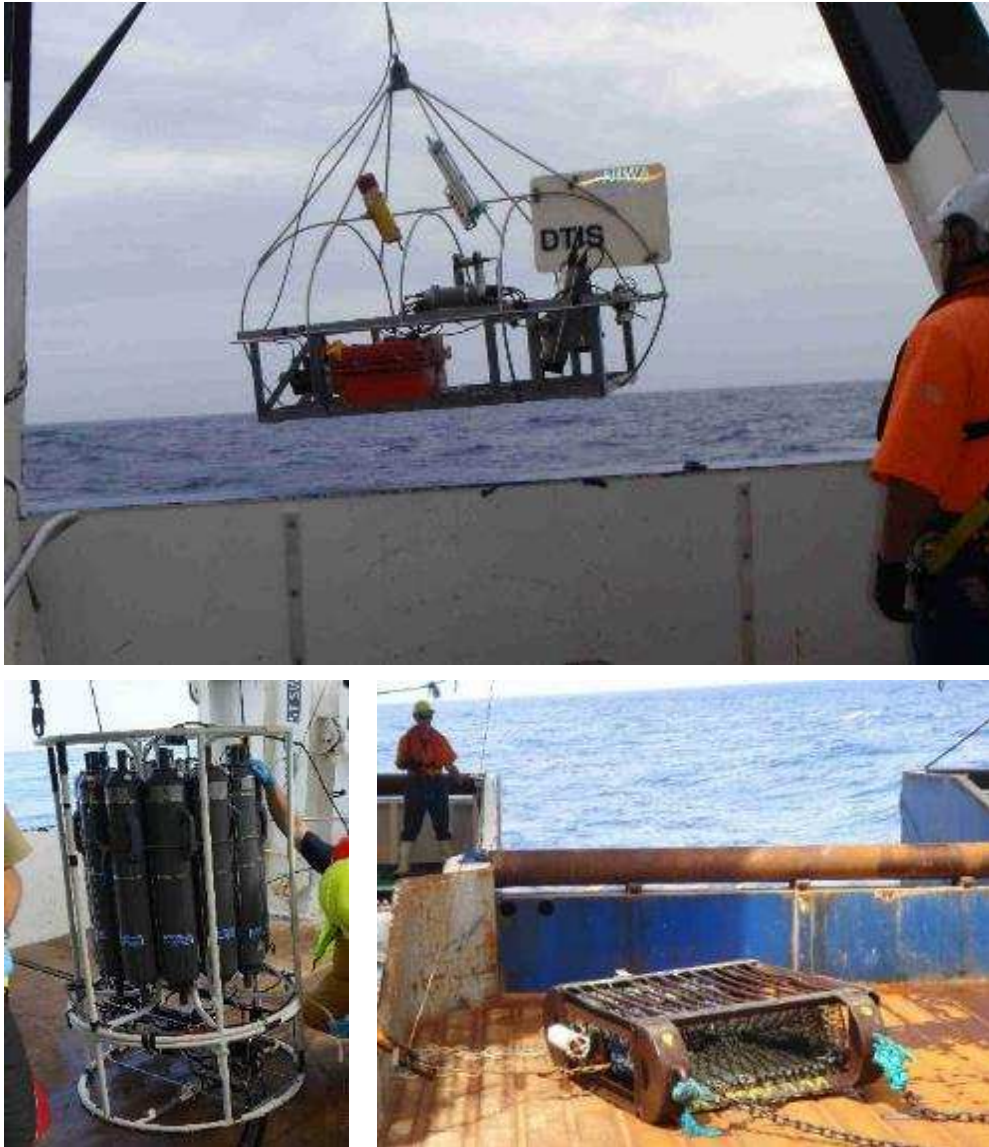
Figure 3: The sampling gear used for the survey: DTIS (top), the Seamount sled (lower right), and 12 bottle CTD (lower left).
