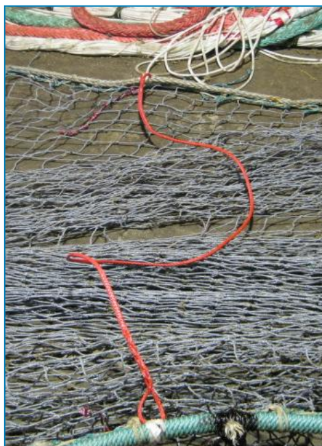
Nylon braid restrictor fitted
