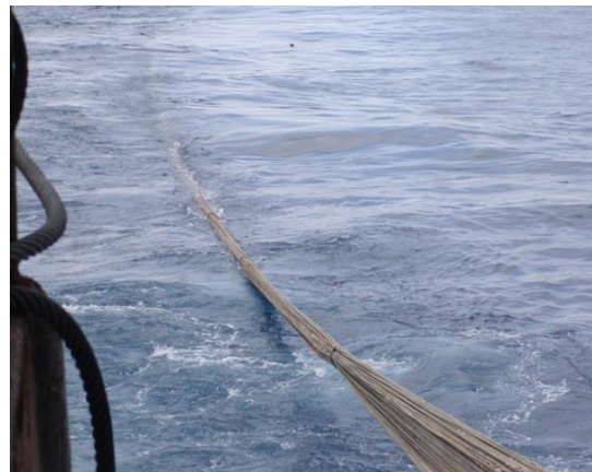
Fig 2: Trawl shot away with net binds
