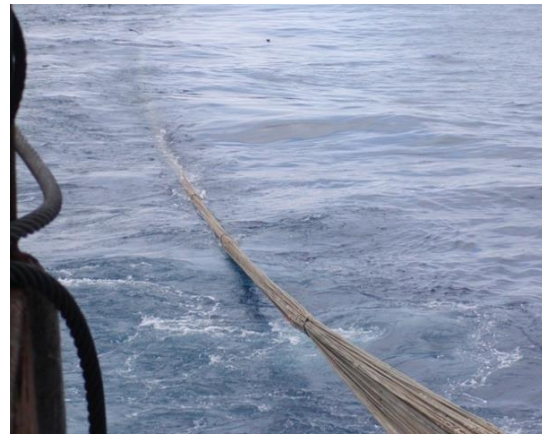
Fig 2: Trawl shot away with net binds
