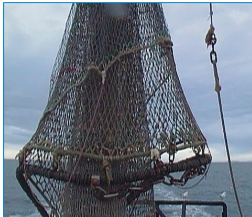
Trawl with restrictors
