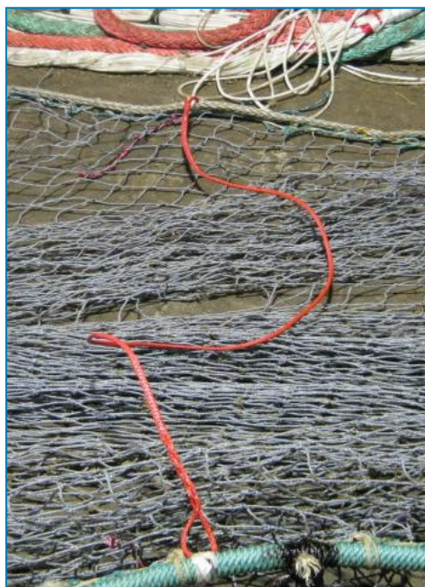
Nylon braid restrictor fitted
